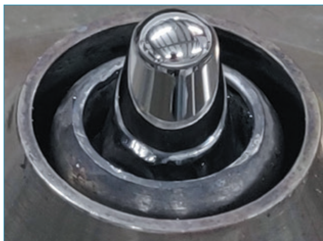
FIGURE 3. An example of a wetted nozzle.
