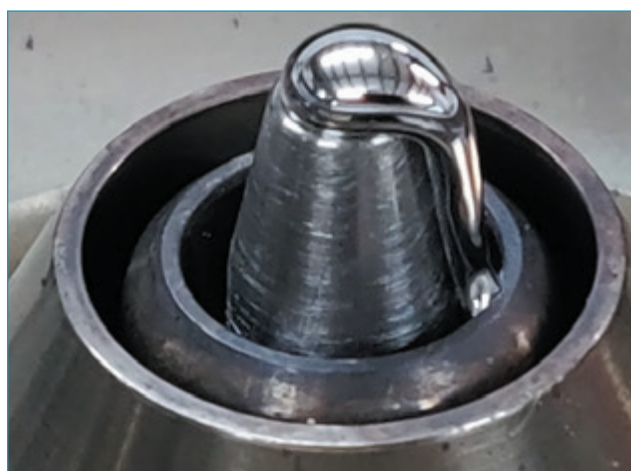
FIGURE 4. An example of a non-wetting nozzle.
