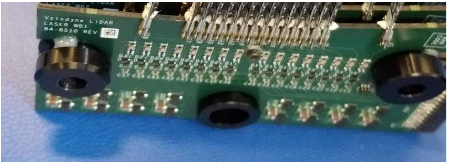
Figure 3. When a collection of eight PCBs has 16 lasers attached to each, the temperature inside the Lidar sensor is bound to rise.
