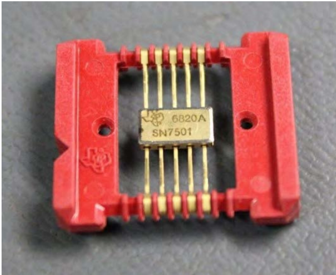
Figure 1. Many of the earliest IC packages, notably those from TI, were flat leaded and surface mounted. This carrier contains 10 ceramic ICs having 10 leads each with soldered lids.
