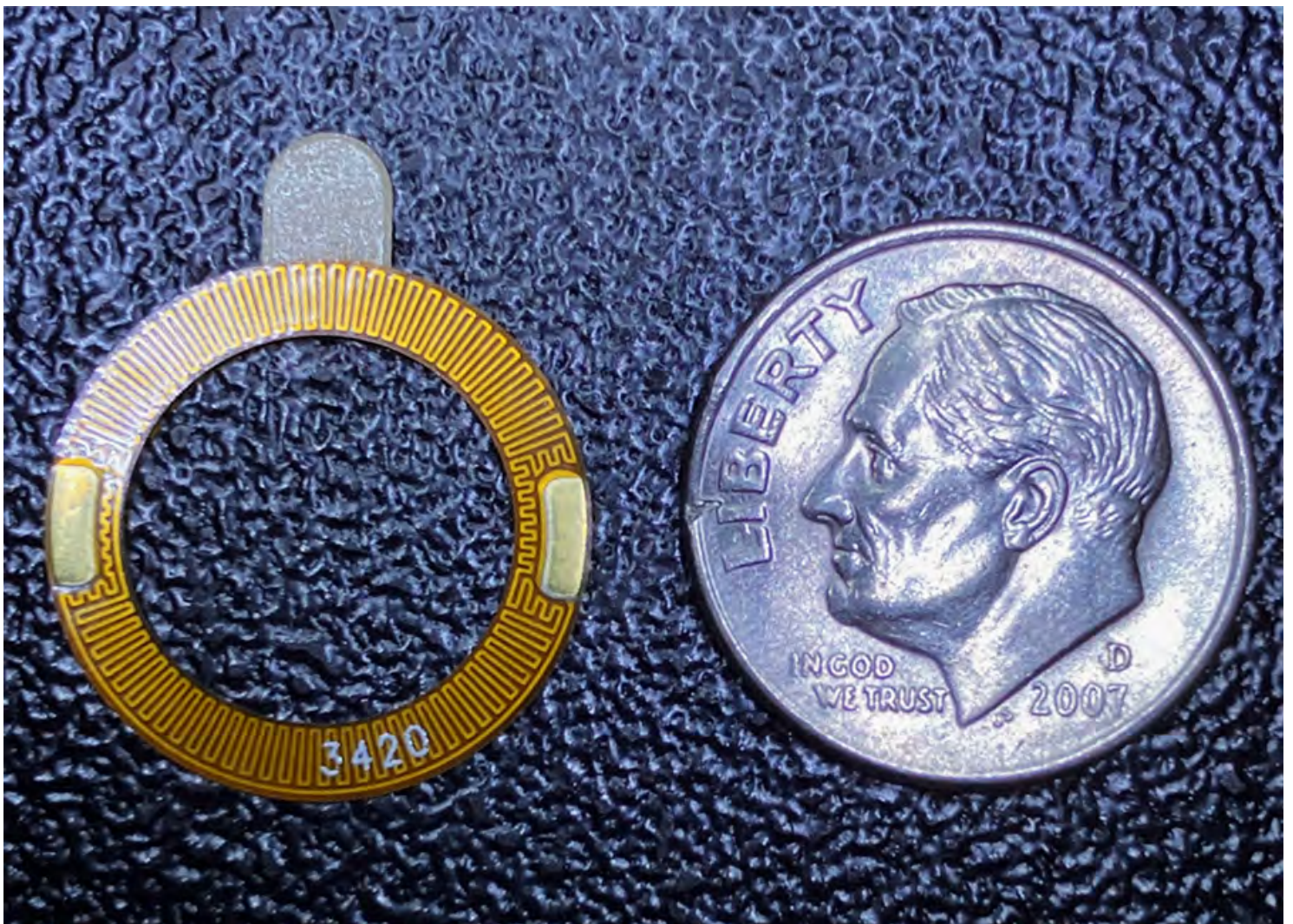
Figure 1. Thin resistive CuNi alloys permit much higher resistance density than copper.
