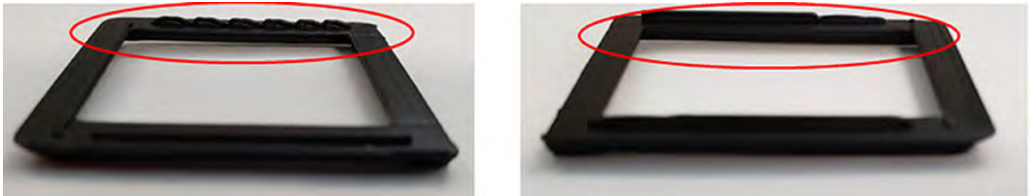
Figure 22. Removed retaining wall structures showing incomplete ABS extrusion into 0.8mm PCB grooves using 0.6mm diameter nozzle.
