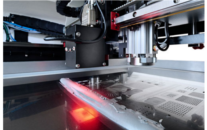
Machine vision on the ii-P7 look-down camera evaluates the entire paste roll length to guard against insufficient paste volume before a print stroke.
