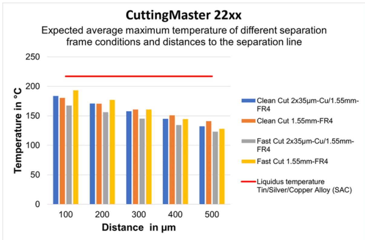
Figure 3. Average maximum temperatures for different cutting strategies, material compositions and distances to the cutting channel.
