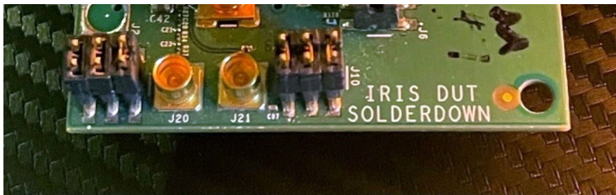
Figure 1. One of many iterations of a test board for a WiFi/Bluetooth/FM combo device in a wafer-level chip-scale package (Source: Author).
