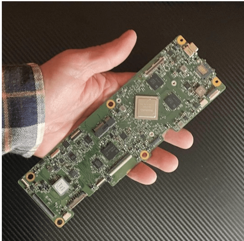
A six-layer board that uses the outer layers for routing as well as placement. (Image credit: Author)
