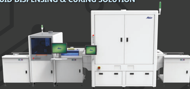
Loading >> Dispensing >> Inspecting >> Curing >> Unloading
