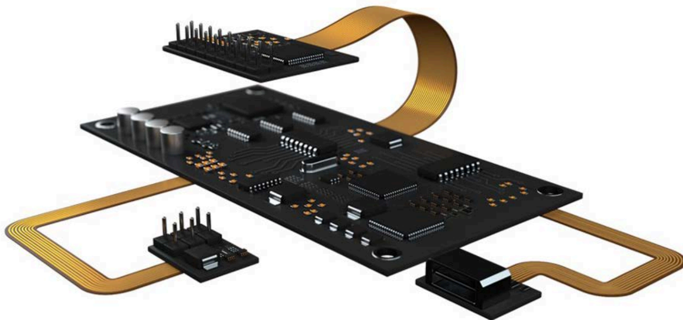
Figure 3. The options are endless with segmenting electronics over rigid-flex designs. (Source: Cadence)
