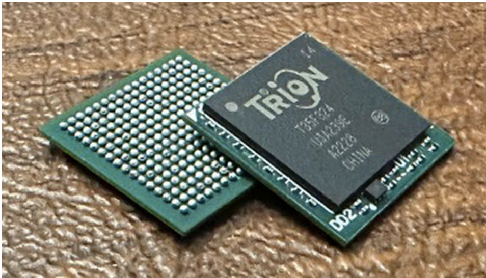
Figure 2. PCB interposers can provide a solution to semiconductor obsolescence or unavailability.
