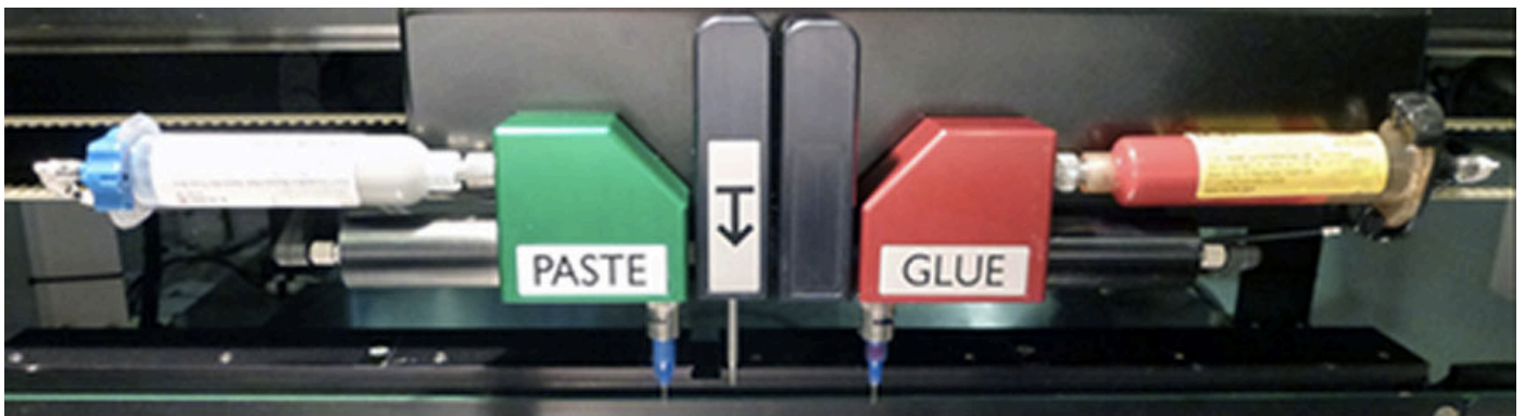
Figure 2. A solder paste dispenser mounted inside a stencil printer.
