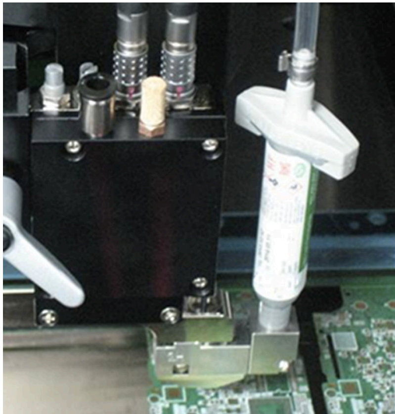
Figure 3. A jet dispenser on an SPI system touches up insufficient paste deposits and then reinspects to ensure proper volume.
