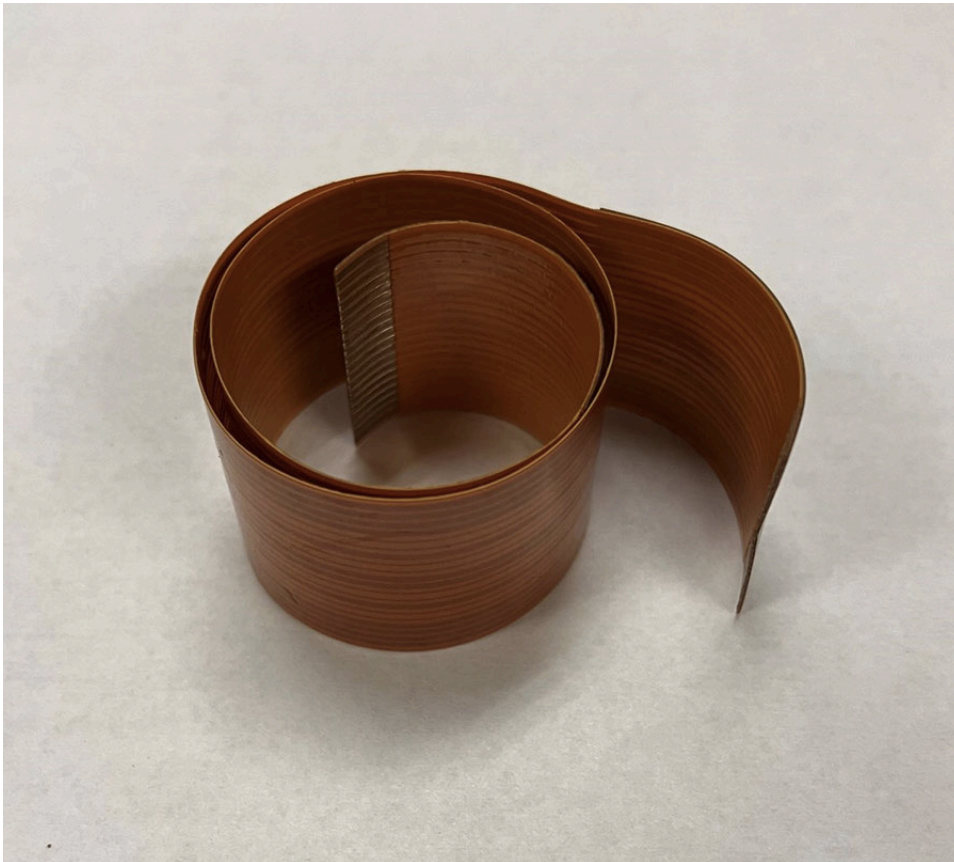
Figure 1. Clock spring flex-circuit designs can help facilitate electrical connections to rotating features in an electromechanical assembly.
