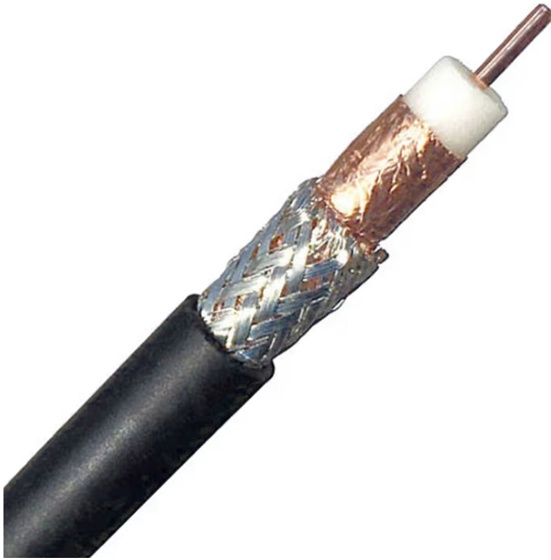
Figure 1. A coaxial cable creates a Faraday cage around the central conductor. The isolation and controlled impedance permit much longer runs without signal degradation. (Source: BHPhotoVideo)
