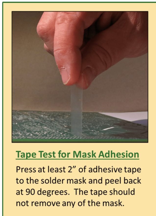
Figure 1. Tape test for solder mask adhesion.
