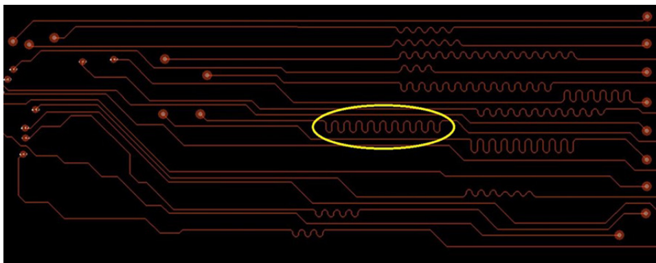
Figure 12. Adding serpentine traces to match line lengths.
