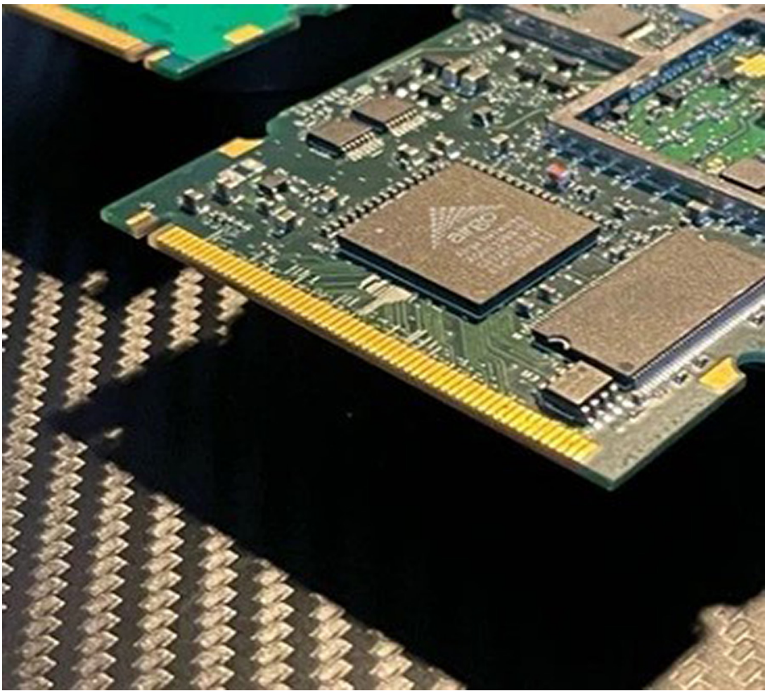
Figure 2. A PCIe mini edge card connector. The PCB thickness is standardized on 0.8mm, requiring its own class of fine-pitch connectors.
