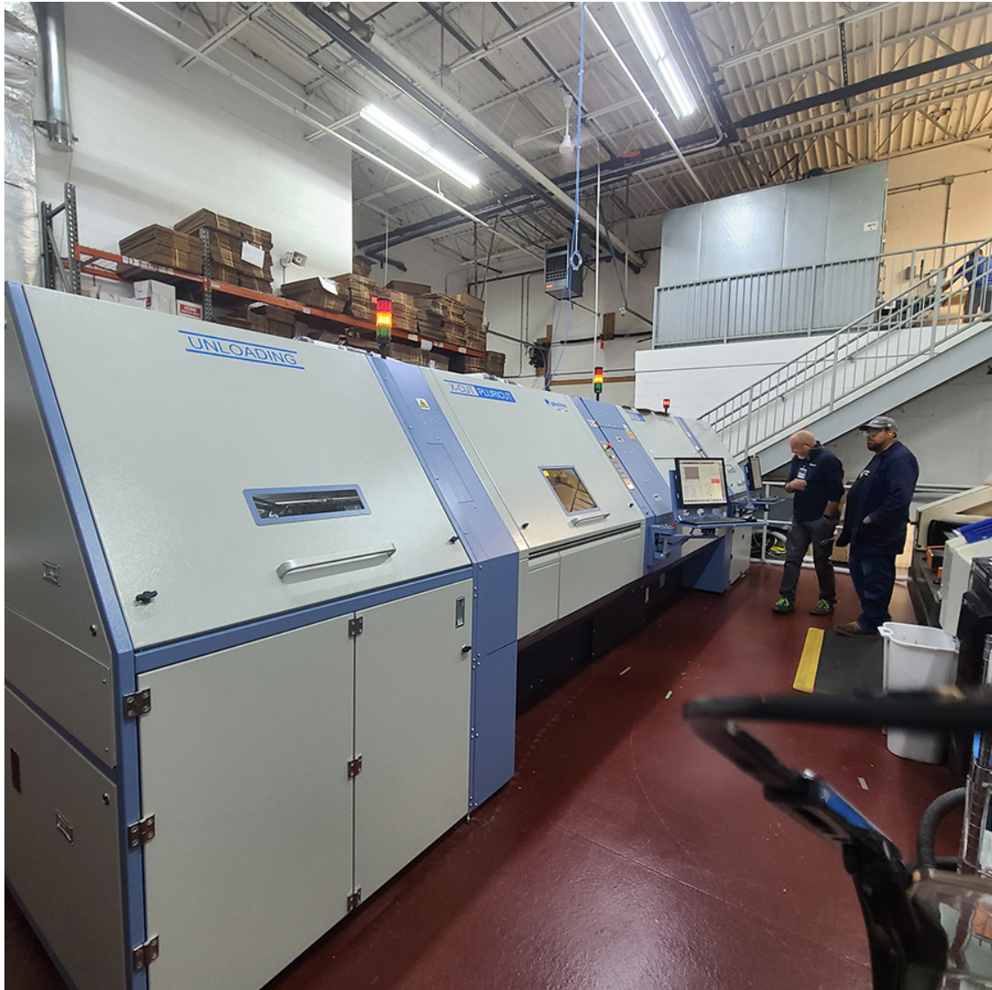
Figure 2. The West Chicago plant's new Pluritec X-Cut S1 drill and bar coder.
