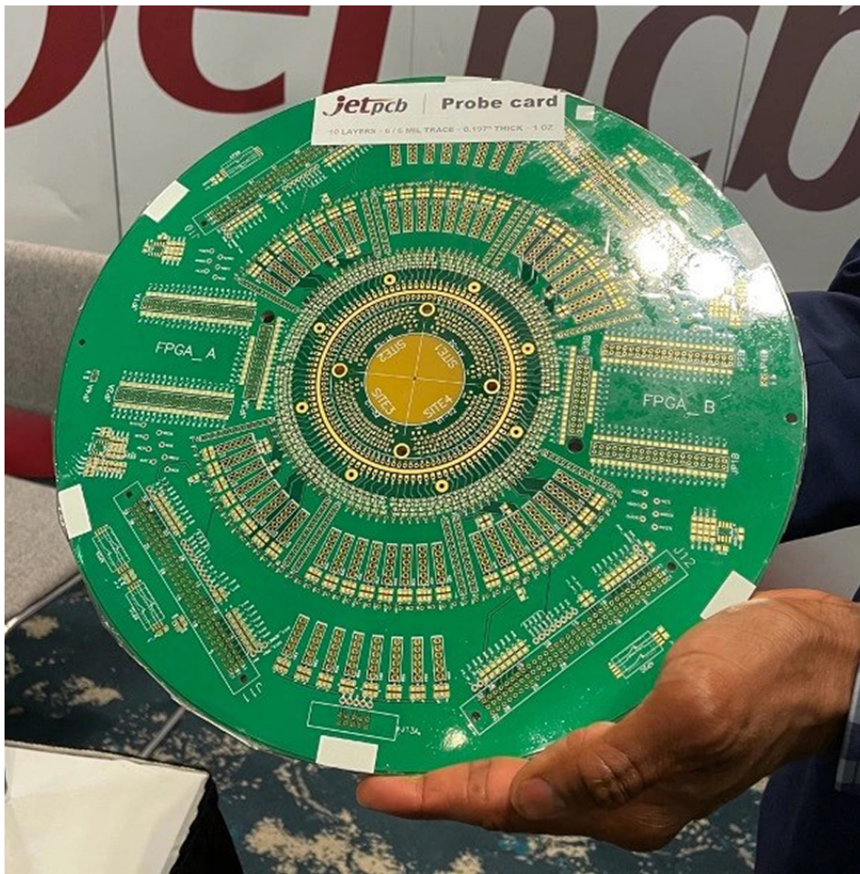
Figure 2. Get the chip team's attention with probe cards that help them quantify the device's throughput.
